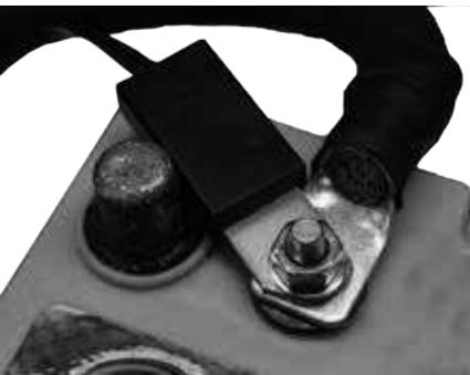
Fig 2.5(b) Temperature Sensor Installation
