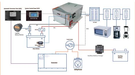
Installation is critical and starts with an analysis of the electrical system's size and power usage in order to understand how the owner will use the inverter. That information is important in specifying the right size of inverter to put on the boat.
