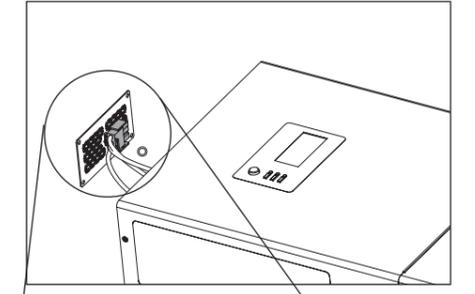
Cut the cable tie holding the unit's GFCI connector **C** to the GFCI cover plate **B**.
