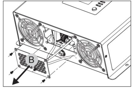
Remove the four screws and detach the GFCI cover plate **B** from the inverter unit. Set aside the screws.
