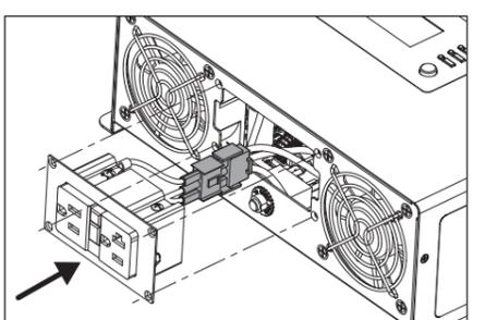
Mount the GFCI device onto the inverter unit.
