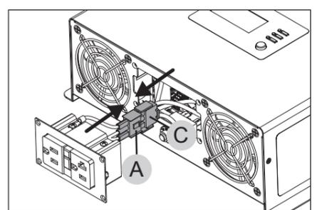
Attach the two connectors together **A** → **C**.
