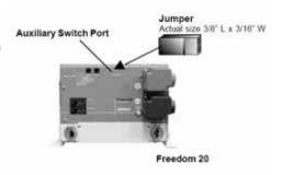
Current versions of the product do not require the installation of the jumper, because it is no longer necessary for operation of the inverter when used without a remote control. The Auxiliary Switch Port can now be used to turn the inverter on with the use of a contact closure. Connecting these two pins together turns the inverter on, and disconnecting them turns the inverter off. Some RV manufacturers use this feature to power a back-up camera and a 120 Volt TV.
