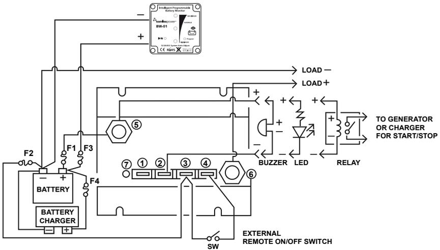
Fig 5.1 Connection Diagram for BG-200
