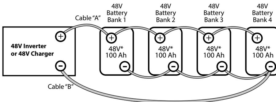
\* **NOTE:** Each of the 48V, 100 Ah battery banks will consist of (i) 8 pieces of 6V, 100 Ah batteries in series or (ii) 4 pieces of 12V, 100 Ah batteries in series.
