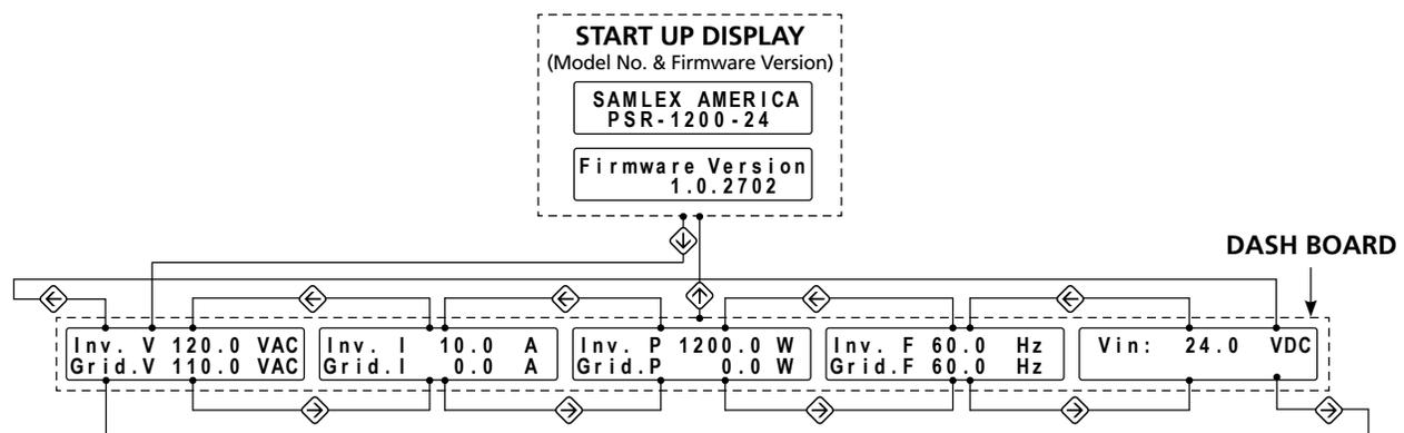
Fig 9.1: Startup Display and Dashboard (extract from Fig 10.1)
