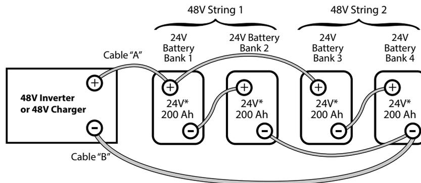
\* NOTE: Each of the 24V, 200 Ah Battery Banks may be (i) 2x 12V, 200 Ah batteries in series, or (ii) 4x 6V, 200 Ah batteries in series
